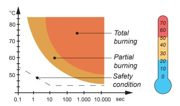
The graph at the side of text indicates the degree of burning that can be caused depending on water temperature and heat exposure time. The mixer solves this problem by interrupting the flow of hot water when the flow of cold water is missing at the inlet.
