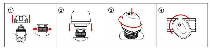
Remove the withe cap on the valve or on the insert of the manifold bar. Install the quickcoupling system on the insert and screw the ring to its end. Tighten the actuator on the locking nut with the aid of the dowels. While holding down the actuator towards the quickcoupling system, turn it clockwise until it stops To remove the electrothermic actuator from the quickcoupling system, simply turn it counter clockwise
