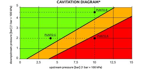
furthermore, to avoid that the ratio between the maximum pressure upstream and the regulation pressure downstream of the reducer exceeds the value of 2.5
